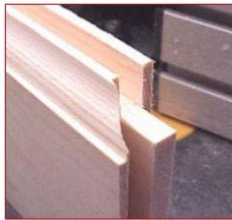
Figure 1: Using a Backer Board to Prevent Tear-Out
