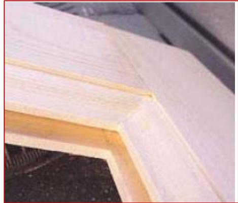
**Note:** Any variation in thickness between the work pieces is shifted to the rear because both the rails and stiles are machined face down. Corrective sanding does not affect the profiles.
